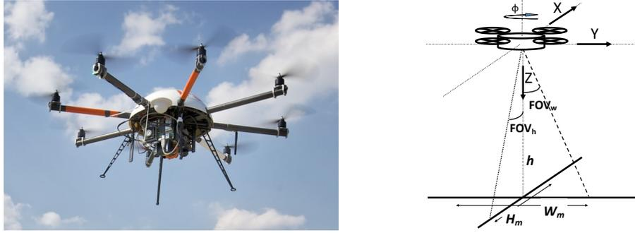
**Fig. 1.** The employed UAV octo-copter platform (left); and a schematic of the UAV hovering over the ground plane. The two FOV angles are depicted, as well as the UAV coordinate system, and  $W_m$  and  $H_m$  ground distances (right).
