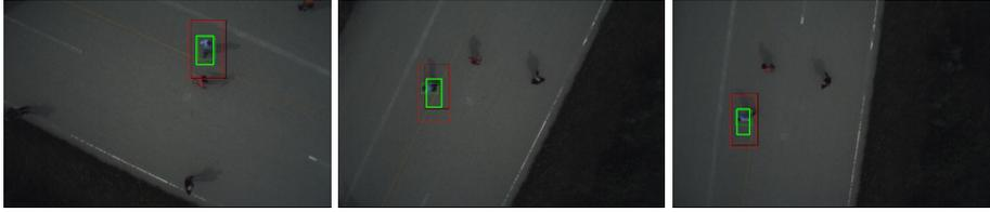
**Fig. 2.** Frames 2220, 2240, and 2260 from the ‘blue’ sequence. In 40 frames, the UAV undergoes a severe rotation about the  $Z$  axis. The proposed method successfully tracks the target (green) with a reduced search window size (red).
